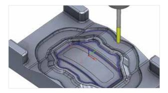
The SolidCAM HSM module features several enhancements to CAM technology that make high speed operations possible, including avoiding sharp angles in the tool path, ensuring that the tool stays in contact with the part as much as possible, and optimizing non-machining moves to reduce air cutting and generating smooth and tangential lead in/out.
