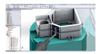
For controllers with advanced plane rotation or coordinate rotation functions, SolidCAM's post processors are configured to use these internal CNC functions. If you have a machine without such functions, users can input the part location inside SolidCAM and the G-code will handle all of the transformations for each rotation.
