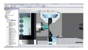
The fastest growing and most demanding class of CNC machines on the market today are multi-task machines that combine several capabilities into one machine – multiple spindles, multiple turrets, material being machined in multiple stages, transferring from spindle to spindle without handling, stock inserted at one end, finished parts coming out the other.
