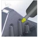
This will maintain the optimum contact point between the tool and the part and enables the use of shorter tools for more stability and rigidity.
