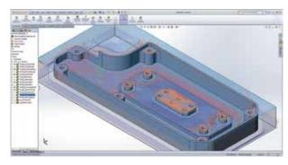
The unique Technology Wizard provides optimal feeds and speeds, taking into account the toolpath, stock and tool material as well as machine specifications.
